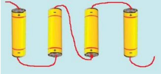
**4. The bulb in the circuit shown in Fig.14.23 does not glow. Can you identify the problem? Make necessary changes in the circuit to make the bulb glow.**
